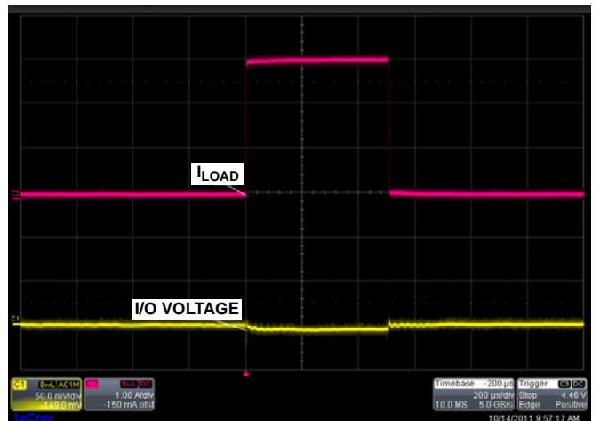
FIGURE 10. I/O VOLTAGE 1.5A LOAD TRANSIENT RESPONSE
